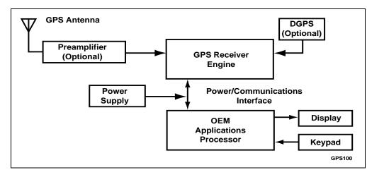
Figure 4. Typical "Jupiter"/OEM Architecture
