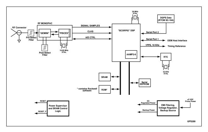
Figure 3. "Jupiter" Receiver Architecture
