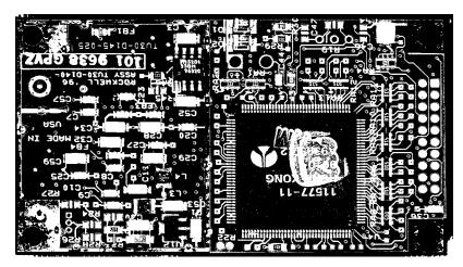
Figure 2. The Rockwell "Jupiter" GPS Receiver (Bottom View -- Shown Approximately Twice Actual Size)
