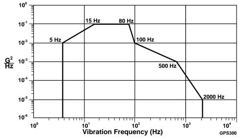
Figure 5. SAE Composite Curve (Random Noise)
