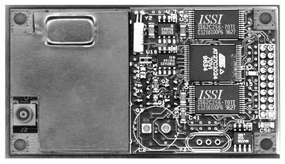
Figure 1. The Rockwell "Jupiter" GPS Receiver (Top View -- Shown Approximately Twice Actual Size)
